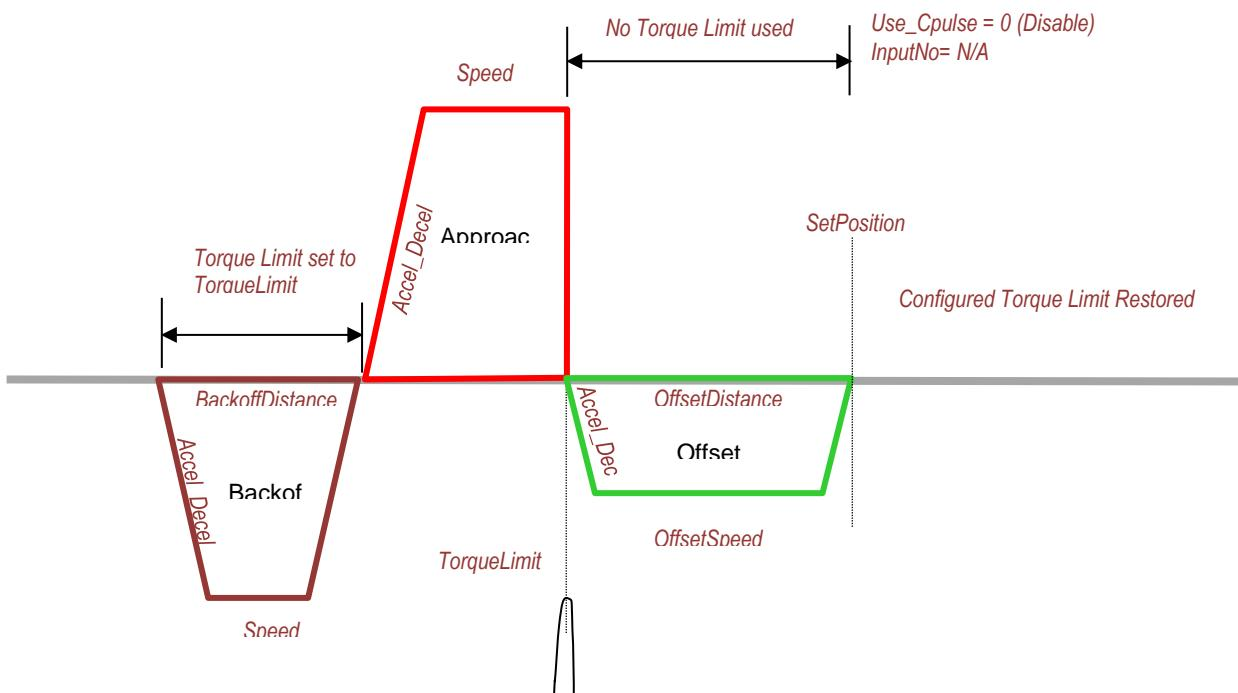
Home to Hard Stop with C-Pulse moves the servo under a Torque Limit until the hard stop is reached according to the following sequence:
